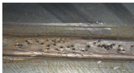
Figure 3 Delineative outline exemplication of linear, cluster porosities in welded pipes [1][3].
