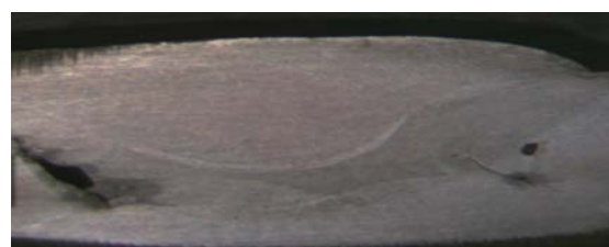
Figure 5 Delineative representation of Lack of Fusion in weld-
